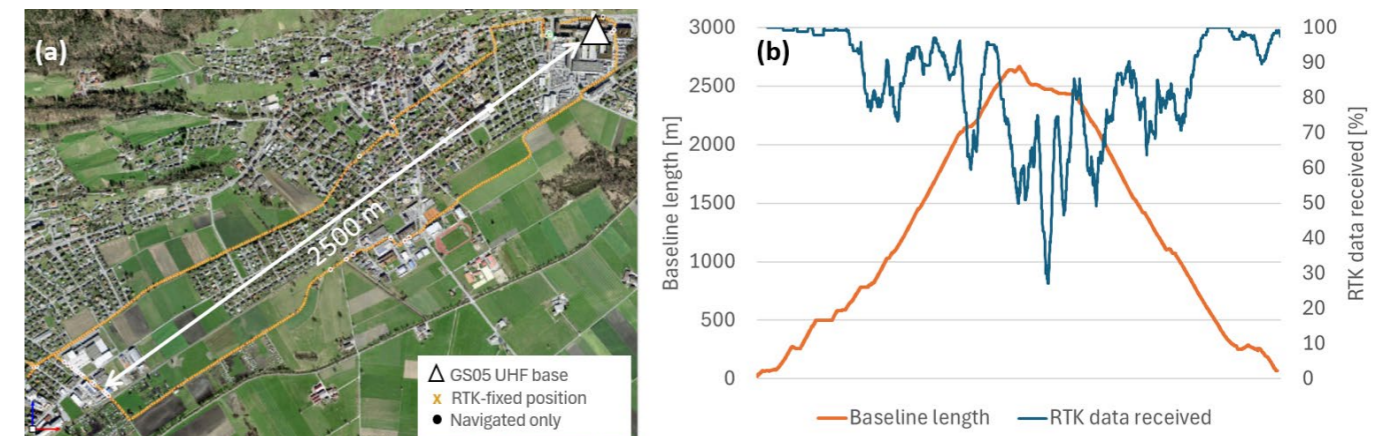
Figure 3: GS05 UHF single baseline range test in Heerbrugg (a) Location and position type overview, (b) Percentage of received RTK data compared to baseline length.
